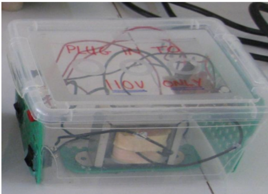
Figure 5: SBPSU with secured cover and warning label indicating only 110V AC input
